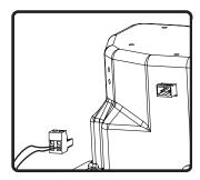
**4.** Connect Euroblock to speaker wires, and connect to speakers.
